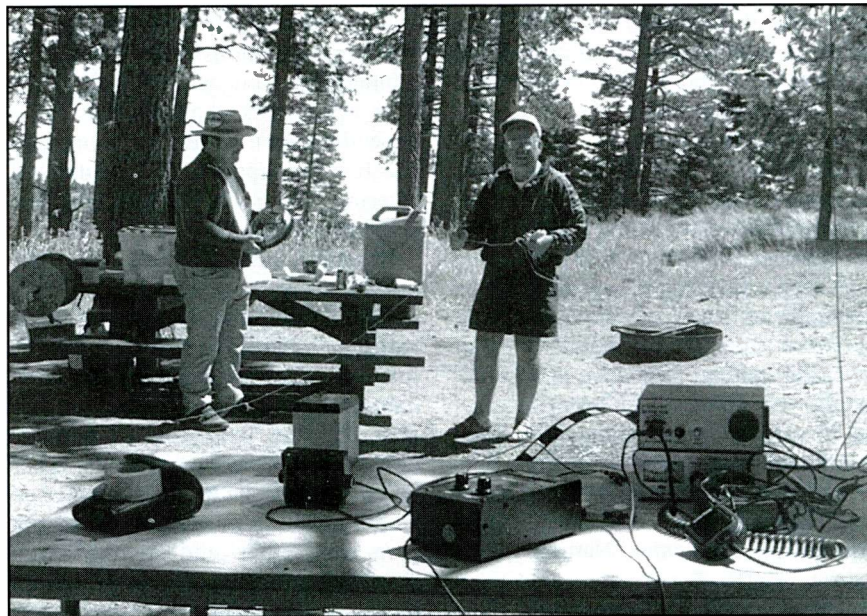
Jerry Parker, WA6OWR, and Doug Hendricks, KI6DS, of the Northern California QRP Club (NorCal) are shown busily erecting a wire antenna prior to Field Day. Note the tiny transceiver sitting atop the MFJ antenna tuner (right center). Low power radios and wire antennas typify Field Day. Unless you try them yourself, you have no idea how effective these low-power radios really are. (K7SZ photo)
