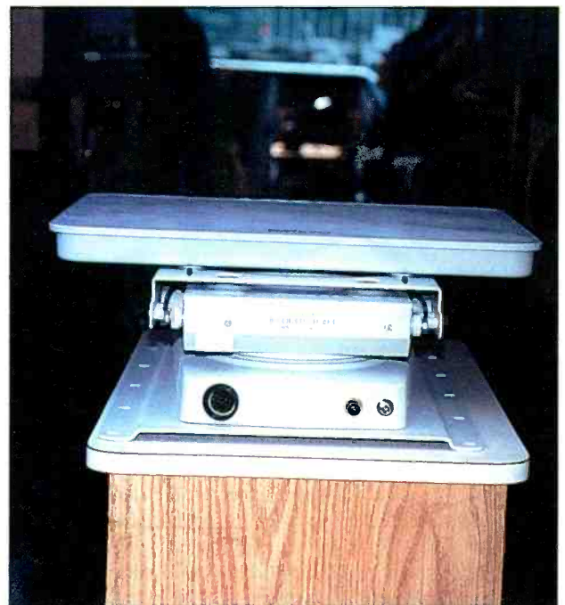
The compact motorized auto-seek flat panel satellite antenna system shown in nested position.
