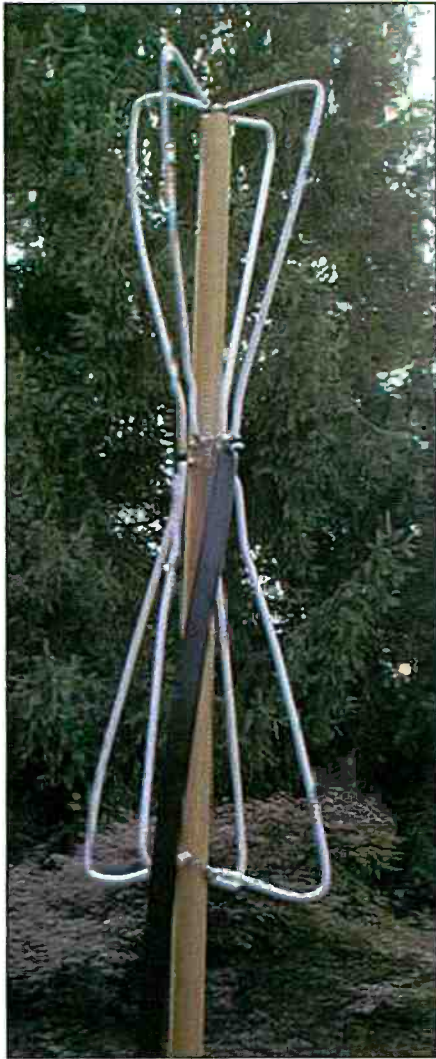
A 360-degree vertical bow-tie antenna.
