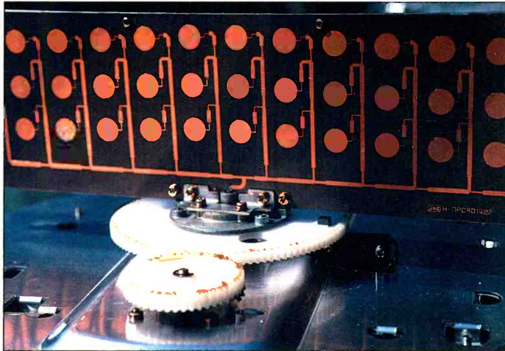
A close up of a phased array circuit board antenna system.
