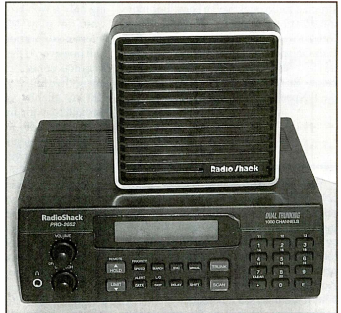
Trunking scanners are available in all shapes and sizes. Here’s a base/mobile unit from RadioShack.
