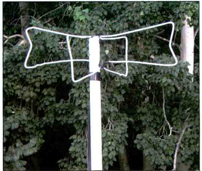
A 360-degree horizontally polarized folded bow-tie dipole antenna.
