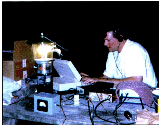
Paul Stroud, AA4XX, avid low-power DXer and contester is pulling the “Night Watch” during the annual ARRL Field Day. The tiny 2.5-watt Wilderness Radio Sierra kit CW transceiver sits atop the antenna tuner just to the right of the computer. DC powered computers are essential for amateur radio FD operations as well as emergency communications scenarios. (K7SZ photo)
