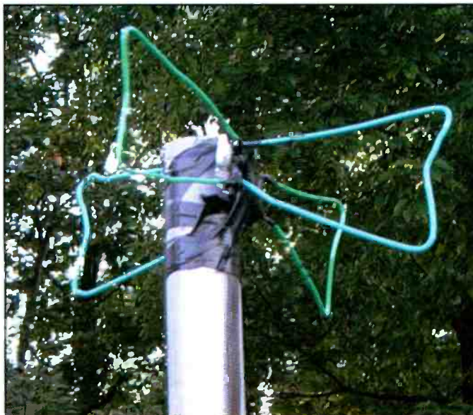
A 360-degree horizontally polarized bow-tie dipole antenna.
